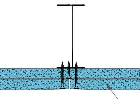
2 layers of 15mm British Gypsum Gyproc SoundBloc fixed with SPEEDLINE Drywall Screws at 300mm centres (200mm centres at external angles). Ref to table for fixing length.
